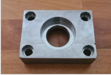
Bearing housing Material – Steel
