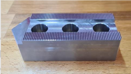
Soft jaw – lathe chuck Material – Steel
